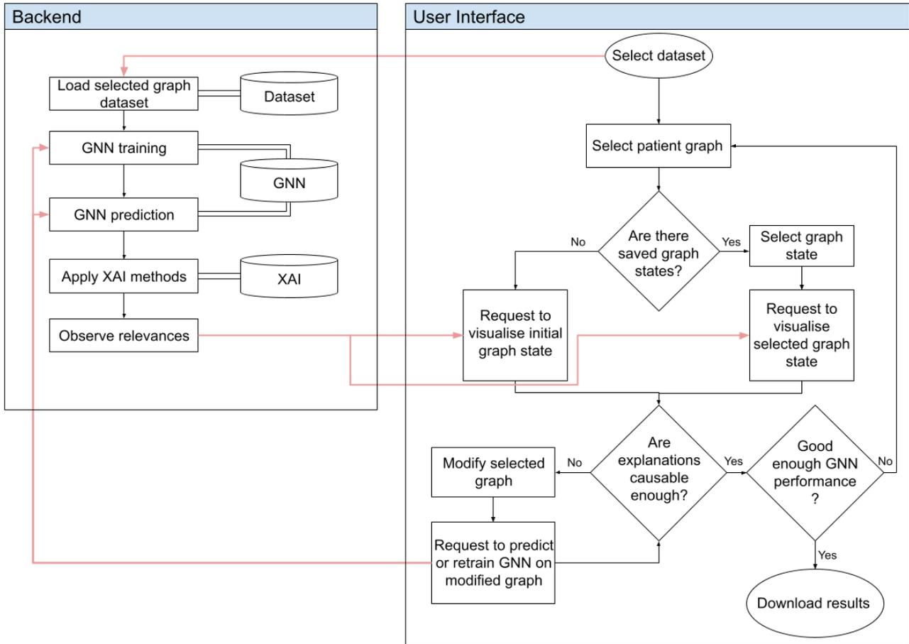
Prediction procedure. The graphs that were changed by the actions of the user are marked with pink colour. After the “predict” procedure is activated (through the pressing of the “predict” button) the GNN remains unchanged but the predictions of the changed graphs (in general) change - and therefore their relevances also. The predictions of the unchanged graphs remain intact. This is shown in the following figure.
