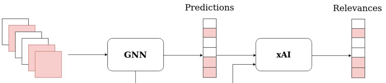
Retrain procedure. The graphs that were changed by the actions of the user are marked with pink colour. After the “retrain” procedure is activated (through the pressing of the “retrain” button) the GNN changes internally, and the predictions of all graphs change - and therefore the relevances also. This scenario presupposes that at least one of the changed graphs belongs to the training set.
